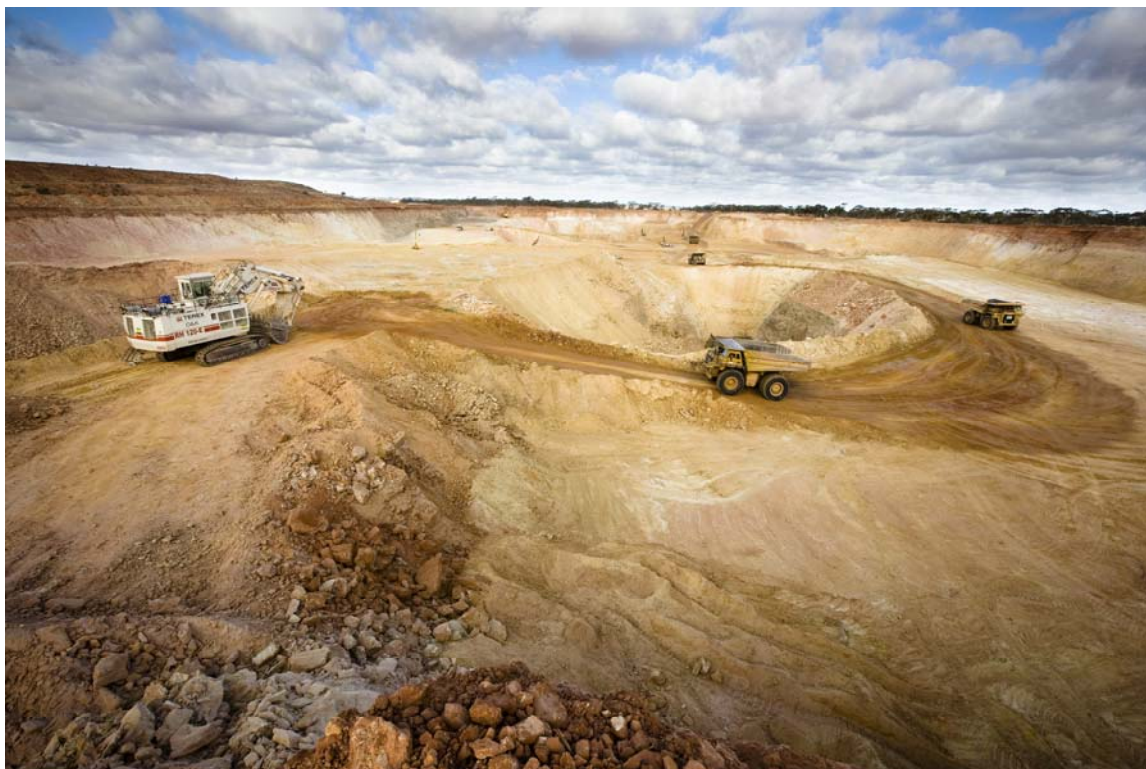
Navajo Chief: Terex RH120 (300 tonne) excavator loading Caterpillar 785 (150 tonne) trucks.
