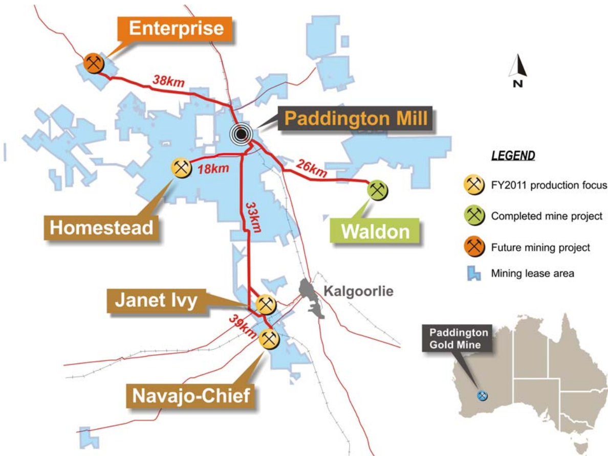
Paddington location map: Paddington mine sites and haul distances to the plant.
