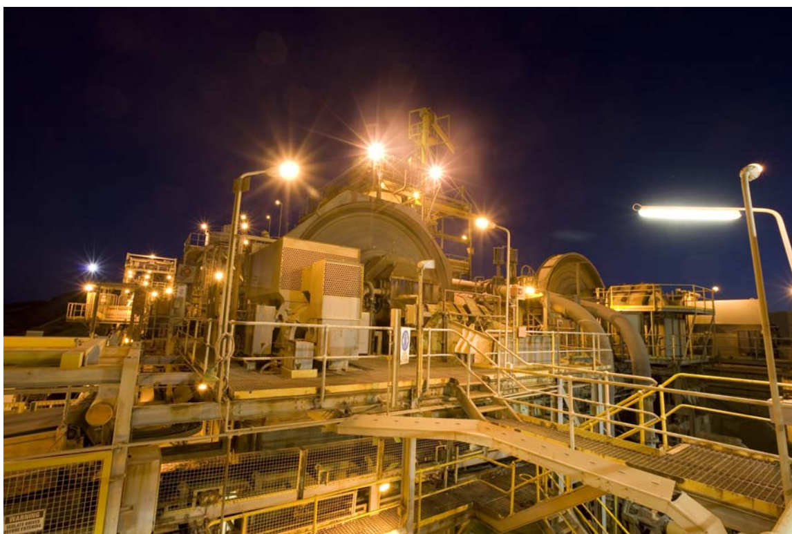
Paddington mill: The 3.3 Mtpa processing plant comprises a primary gyratory crusher, SAG and ball mill, a gravity gold recovery plant and a standard Carbon-In-Leach gold recovery circuit.
